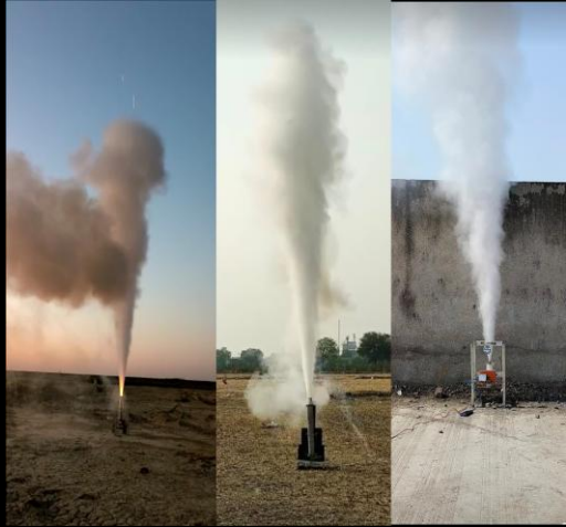
Tested Re-usable 2.5kN Solid Rocket Motor
